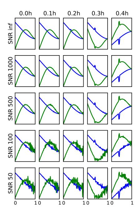
**Figure 4.** POM curvature (first two POMs shown) for damage cases with a crack located at 40% of the beam length, cf. Figure 3
