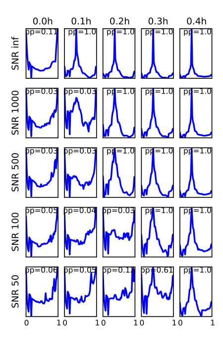
**Figure 3.** Log-marginal likelihood of the model as a function of the parameter  $x_d$ , for various crack depths located at 40% of the length of the beam.
