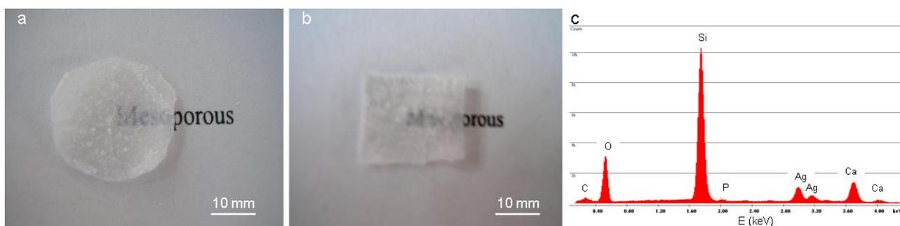
**Fig. 3** - Calcined mesoporous membranes: (a) disk-shaped and (b) rectangle-shaped (“plug”) samples; (c) EDS pattern.
