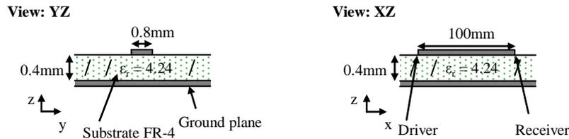
**Figure 3 – Test structure.  $50\Omega$  microstrip track on FR4 substrate of height 0.4mm and track width 0.8mm. The driver inverter feeds the line at  $x$ , and the load inverter is placed at  $x + 100$ mm.**
