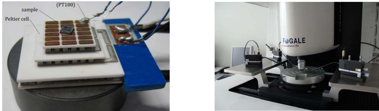
Figure 2. Experimental set-up with Peltier Cell Fogale® and Zoom Surf 3D Fogale® (courtesy of Lab. Design and characterization of microsystems– Politecnico di Torino).
