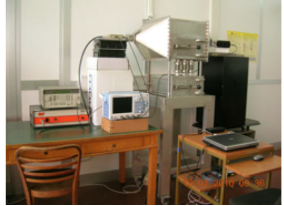
Fig. 7. TEM cell: (a) block diagram of the measurement system, and (b) experimental setup.
