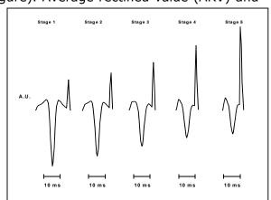
EXAMPLE OF MONOPOLAR POTENTIALS FOR DIFFERENT SHORTENING LEVELS (RELAXED, 13.3%, 26.7%, 40%, 46.6%), FOR A FIBRE UNDER THE DETECTION ELECTRODE (PLACED BETWEEN THE INNERVATION ZONE AND THE TENDON), 6.25 MM DEEP AT THE TENDON LEVELINTO THE MUSCLEE.
