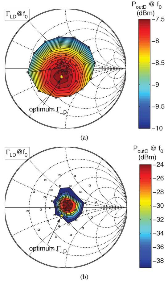
Fig. 5. TC226 differential-mode load map at the fundamental. Shown are the output powers at 1-dB compression of the differential-mode gain. (a) Differential-mode output power versus  $\Gamma_{LD}$ . (b) Common-mode output power versus  $\Gamma_{LD}$ .
