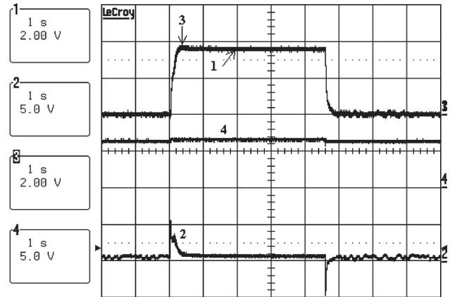
Fig. 5. Drive response to speed step command 0 ÷ 0.36 per unit (10 V/1 per unit). (1)  $\hat{\omega}_r$  (in per unit). (2)  $i_{qs}$  (in per unit). (3)  $\omega_r$  (in per unit). (4)  $\hat{\lambda}_r$  (in per unit).
