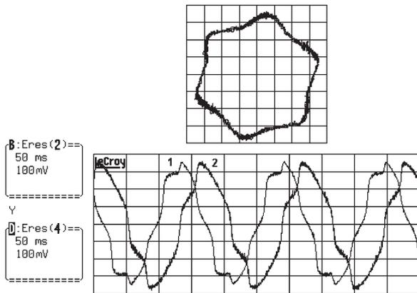
Fig. 15. Stator command voltage components and voltage vector locus in stationary reference frame at low speed ( $10 \text{ V/1}$  per unit) without dead-time compensation. (1)  $v_{s\alpha}^*$  (in per unit). (2)  $v_{s\beta}^*$  (in per unit).
