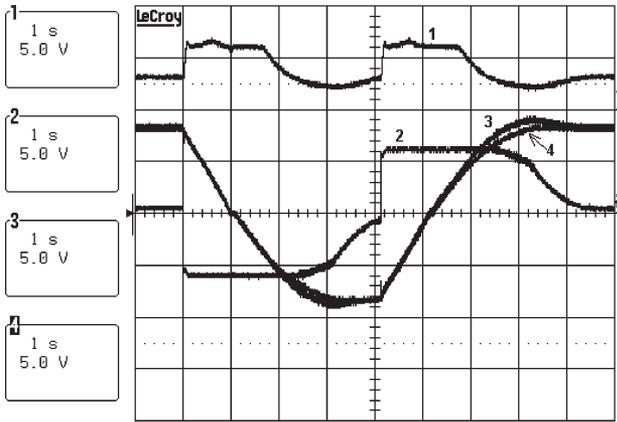
Fig. 13. Speed reversal from  $-0.8$  to  $0.8$  per unit ( $10 \text{ V/1}$  per unit). (1)  $\hat{\lambda}_r$  (in per unit). (2)  $i_{qs}$  (in per unit). (3)  $\hat{\omega}_e$  (in per unit). (4)  $\hat{\omega}_r$  (in per unit).
