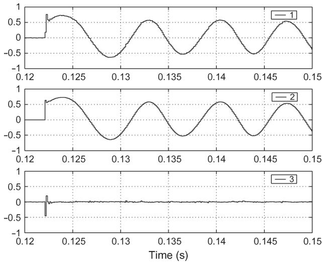
Fig. 8. Measured and estimated  $\beta$ -axis currents at startup. (1)  $i_{s\beta}$  (in per unit). (2)  $\hat{i}_{s\beta}$  (in per unit). (3)  $\varepsilon_\beta = i_{s\beta} - \hat{i}_{s\beta}$  (in per unit).
