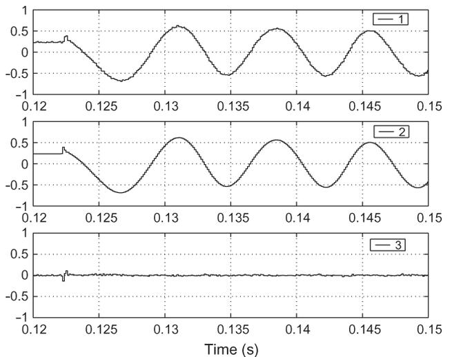
Fig. 7. Measured and estimated  $\alpha$ -axis currents at startup. (1)  $i_{s\alpha}$  (in per unit). (2)  $\hat{i}_{s\alpha}$  (in per unit). (3)  $\epsilon_\alpha = i_{s\alpha} - \hat{i}_{s\alpha}$  (in per unit).
