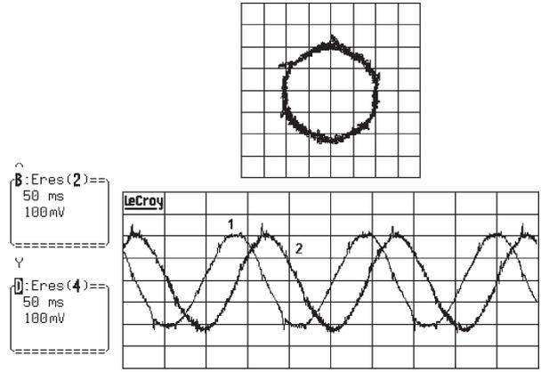
Fig. 16. Stator command voltage components and voltage vector locus in stationary reference frame at low speed ( $10 \text{ V/1}$  per unit) with dead-time compensation. (1)  $v_{s\alpha}^*$  (in per unit). (2)  $v_{s\beta}^*$  (in per unit).
