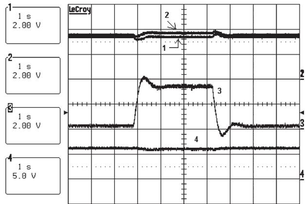
Fig. 11. Load rejection behavior at the limit of constant torque region (10 V/I per unit). (1)  $\hat{\omega}_r$  (in per unit). (2)  $\hat{\omega}_e$  (in per unit). (3)  $i_{qs}$  (in per unit). (4)  $\hat{\lambda}_r$  (in per unit).
