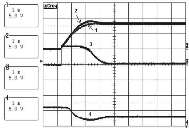
Fig. 12. Drive startup with inertial load up to 0.8 per unit (3100 r/min). (10 V/I per unit). (1)  $\hat{\omega}_r$  (in per unit). (2)  $\hat{\omega}_e$  (in per unit). (3)  $i_{qs}$  (in per unit). (4)  $\hat{\lambda}_r$  (in per unit).
