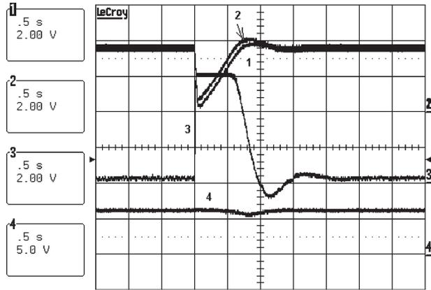
Fig. 14. Short step load change higher than the maximum motor torque. ( $10 \text{ V/1}$  per unit). (1)  $\hat{\omega}_r$  (in per unit). (2)  $\hat{\omega}_e$  (in per unit). (3)  $i_{qs}$  (in per unit). (4)  $\hat{\lambda}_r$  (in per unit).
