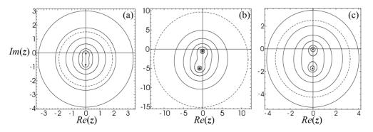
FIG. 4. Plot in the complex plane of spectra (dots), pseudospectra (solid lines), and numerical range (dashed line). The parameters of the contours from the inner to the outer are  $\epsilon = [0.05, 0.10, 0.25, 0.5, 1, 2]$ . S = 1, D = 1.025,  $n_2 = 1$ , F = 0.01, k = 0.1, and R = 30. (a)  $n_1 = 1$ , Z = 0.5, (b)  $n_1 = 4/3$ , Z = 0.5, (c)  $n_1 = 1$ , Z = 0.25. Notice the different scales adopted in the panels.
