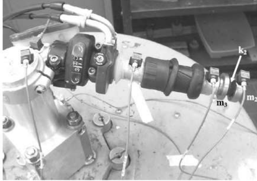
Fig. 9 The handle with the proposed vibration absorber
