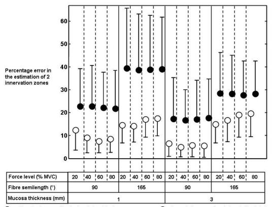
Error between estimated and simulated amplitude IZ distribution
