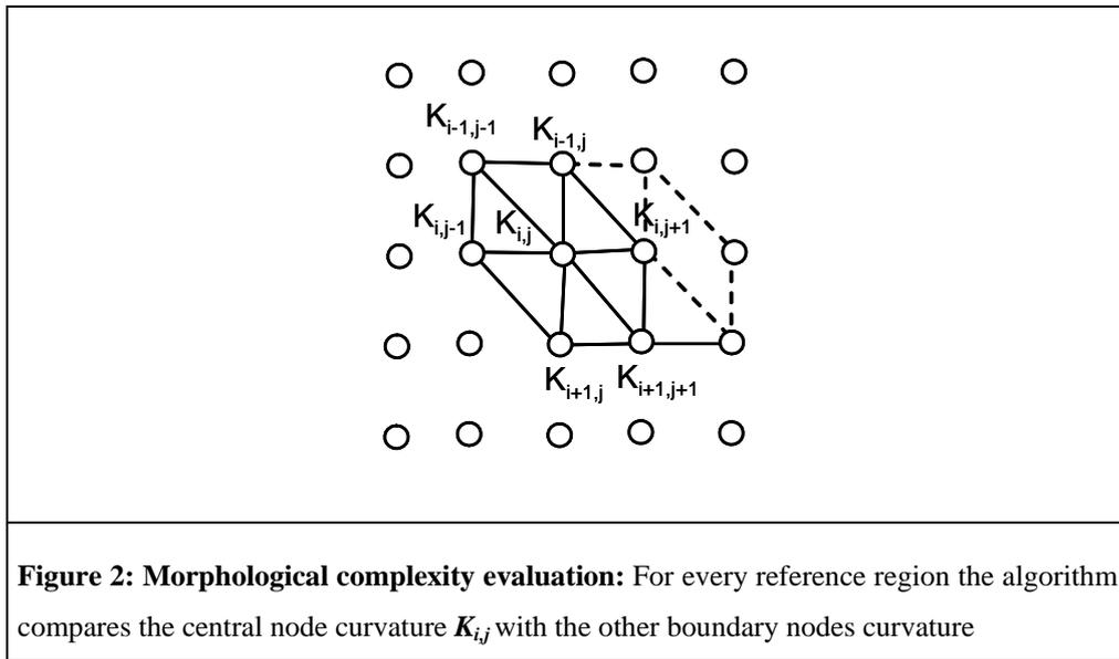
**Figure 2: Morphological complexity evaluation:** For every reference region the algorithm compares the central node curvature  $K_{i,j}$  with the other boundary nodes curvature
