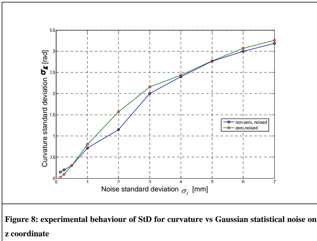
In order to get a mean relation between curvature  $K$  standard deviation  $s_K$  and the known Gaussian noise standard deviation  $s_I$ , which has been just represented (Fig. 8), it has been necessary to identify a model
