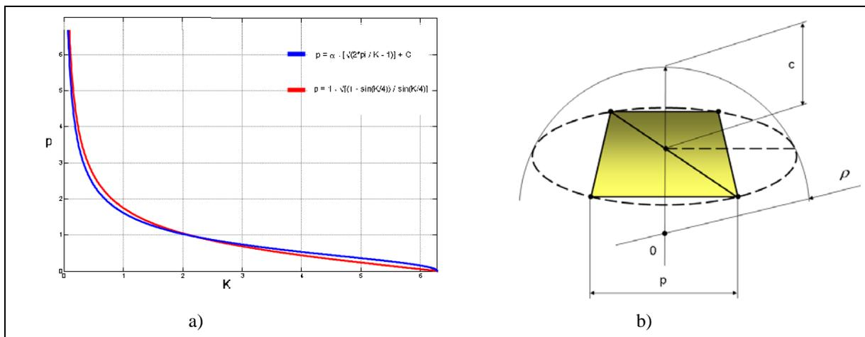
**Figure 15: “Total Deviation Filter”; a) comparison between the pitch Function obtained through the application of a “Total Deviation” threshold (blue), and that represented also by Eq.14, derived from local Curvature Analysis; b) “Total Deviation” Approach; c represents the Deviation amount, between the original Surface (white) and the approximating triangulation (yellow)**
