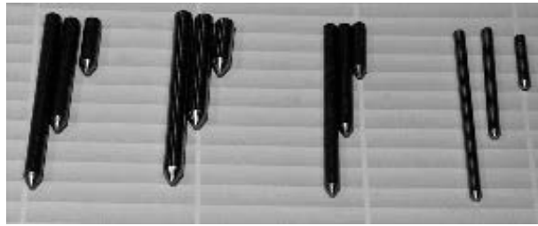
Figure 5: Steel cylinders employed for runners imprinting.
