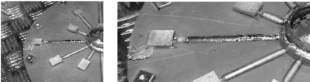
Figure 7: Non controlled material escape and incomplete figure filling.
