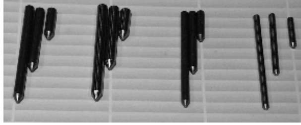
Figure 5: Mould preparation with the use of steel prismatic figures for masters and steel cylinders for runners
