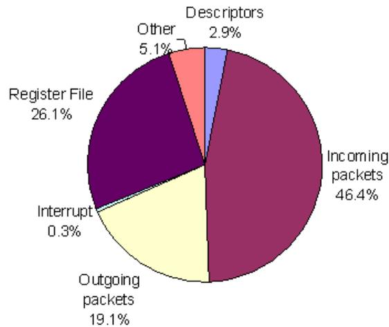
Fig. 8. HERO resource usage break down by function
