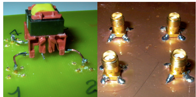
Fig. 1. Test fixture for the measurement technique proposed in this paper. Top panel: device; bottom panel: measurement ports.
