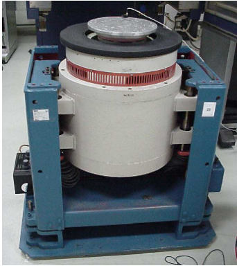
Figure 3. Example of a shaker for CD player test.
