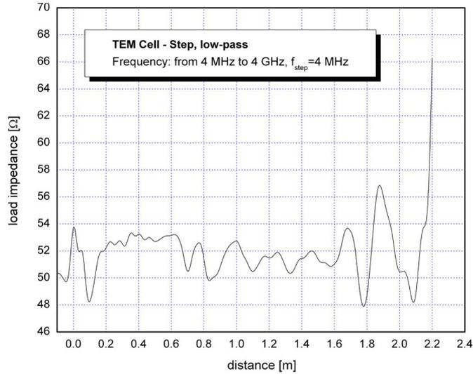
Fig. 5. TDR measurement with VNA: empty TEM cell impedance, low-pass step mode.
