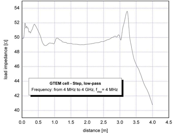
Fig. 3. TDR measurement with VNA: empty GTEM cell impedance, low-pass step mode.
