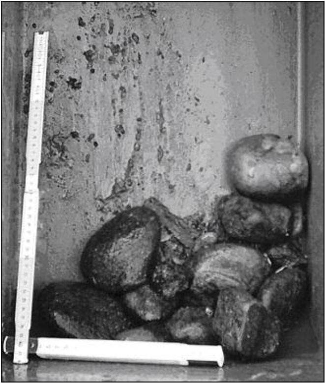
Figure 9 □ Example of coarse riverbed sampled material.
