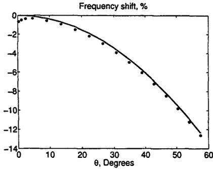
**Figure 5: Percentage frequency shift for the  $2\lambda$  resonance in the differential mode excitation of Type I structure. NEC output (circles) and predicted frequency shift according to the wire lengths (continuous line).**
