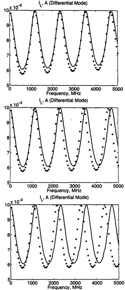
**Figure 4: Type I structure with differential mode excitation. Load current obtained with the NMTL model (continuous line) and NEC (circles) for different divergence angles:  $\vartheta = 9^\circ$  (top panel),  $\vartheta = 27^\circ$  (middle panel),  $\vartheta = 43^\circ$  (bottom panel).**
