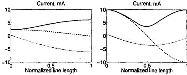
**Figure 3: Current distribution along the active conductor at frequencies corresponding to  $\mathcal{L} = \lambda/4$  (left panel) and  $\mathcal{L} = \lambda/2$  (right panel). Magnitude (continuous line), Real part (dashed line), and Imaginary part (dotted line).**
