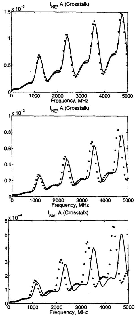
**Figure 6: Type I structure with single conductor excitation. Near-End Crosstalk obtained with the NMTL model (continuous line) and NEC (circles) for different divergence angles:  $\vartheta = 9^\circ$  (top panel),  $\vartheta = 27^\circ$  (middle panel),  $\vartheta = 43^\circ$  (bottom panel).**
