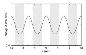
FIG. 2. Schematics of the prototypical 30 Å/30 Å GaAs/Al<sub>0.3</sub>Ga<sub>0.7</sub>As superlattice structure considered in our simulated experiments: Real-space periodic nanostructure profile (shaded regions correspond to barriers) and charge distribution corresponding to the ground-state  $(k_{\parallel}=0)$  envelope function in the field-free case  $[(n(r_{\parallel}) \propto |\phi^0_{k_{\parallel}=0,\nu=1}(r_{\parallel})|^2)]$ .
