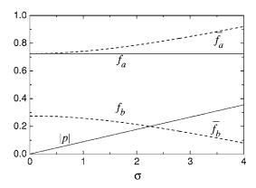
FIG. 1. Phonon-induced single-particle phase coherence for an isolated quantum-dot system: modulus of the interlevel polarization |p| (solid curve) and dressed-states populations  $\overline{f}_b$  and  $\overline{f}_a$  (dashed curves) as a function of the coupling-constant ratio  $\sigma$ , for an interlevel energy splitting  $\Delta\epsilon$ =25 meV at room temperature.
