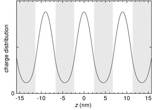
FIG. 1. Schematics of the prototypical 45 Å/45 Å GaAs/Al<sub>0.3</sub>Ga<sub>0.7</sub>As superlattice structure considered in our simulated experiments: Real-space periodic nanostructure profile (shaded regions correspond to barriers) and charge distribution corresponding to the ground-state ( $k_{\parallel}=0$ ) envelope function in the field-free case ( $n(r_{\parallel}) \propto |\phi_{k_{\parallel}=0,\nu=1}^o(r_{\parallel})|^2$ ) (see text).
