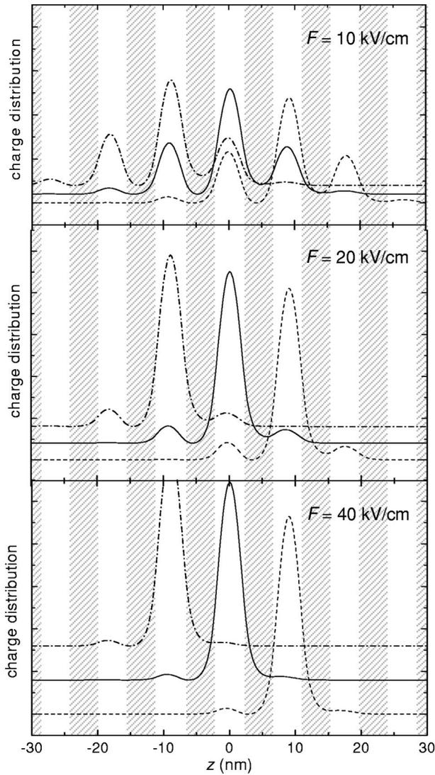
FIG. 3. Charge distribution corresponding to the Wannier-Stark states in the superlattice structure of Fig. 1 for different values of the applied field  $F$ . For each field three states are displayed:  $n = -1$  (dash-dotted curve),  $n = 0$  (solid curve), and  $n = 1$  (dotted curve) (see text).
