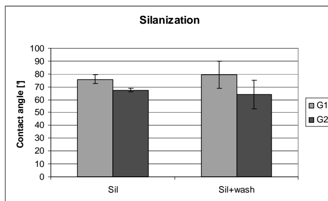
Fig. 1: Contact angle measurement on silanized samples
