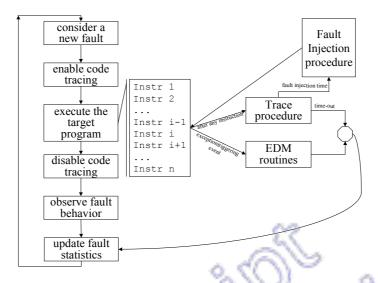
Figure 2: Fault Injection Manager operation flow.
