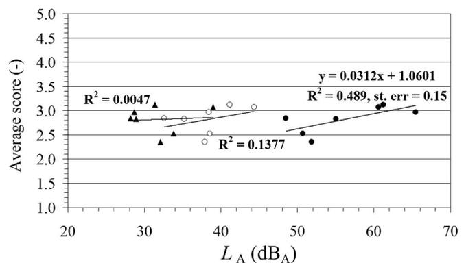
FIG. 5. Average noise disturbance scores versus measured values of  $L_{Aeq}$  (white circles),  $L_{A90}$  (solid triangles) and  $L_{Amax}$  (solid circles) and best-fit regression lines. The five-point scale is bounded by the words "very low" (1) and "very high" (5).
