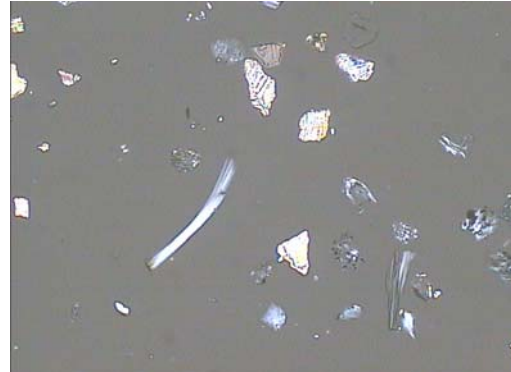
Photo 4. 400 mesh – 20 micrometers class. A partly frayed chrysotile tuft. Short side of the photogram 0,47 mm.
