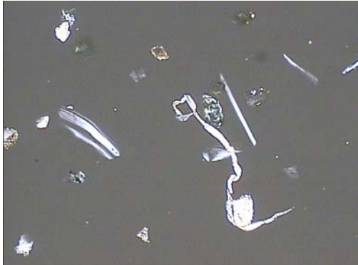
Photo 3. 200 – 400 mesh class. Chrysotile tufts and an organic fibre (at the centre and below). Short side of the photogram 0,94 mm.
