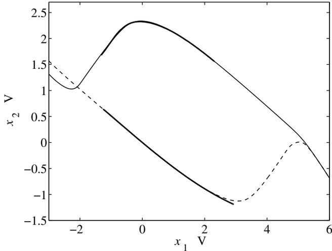
Fig. 6. Static characteristics of submodels  $i_H$  and  $i_L$  in (1) (solid thick curves) superimposed to the actual characteristics of the example driver in fixed high state (solid line) and low state (dashed line).
