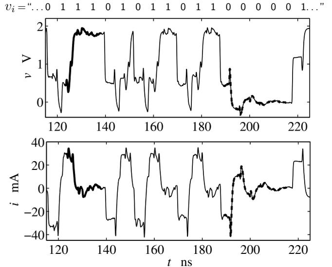
Fig. 5. Output port voltage  $v(t)$  and current  $i(t)$  responses computed for the example driver connected to an ideal transmission line load (characteristic impedance  $Z_0 = 50\ \Omega$ , time delay  $T_d = 2\ ns$ ) loaded by a  $10\ pF$  capacitor. The thick parts of the  $v(t)$  and  $i(t)$  signals are the waveforms used for the estimation of the submodels  $i_H$  and  $i_L$  in (1) (see text for details).
