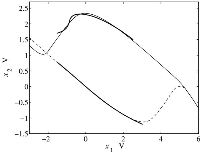
Fig. 9. Static characteristics of the submodels  $i_H$  and  $i_L$  in (1) estimated from noisy signals (solid thick curves) superimposed to the actual characteristics of the example driver in fixed high state (solid line) and low state (dashed line).
