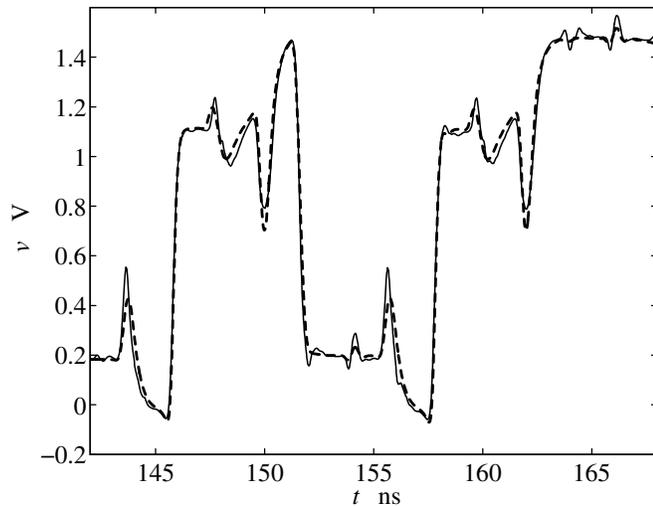
Fig. 10. Port voltage  $v(t)$  response computed for the example driver connected to an ideal transmission line load (characteristic impedance  $Z_0 = 50\Omega$ , time delay  $T_d = 1 ns$ ) loaded by the shunt connection of a  $100\Omega$  resistor and a  $5 pF$  capacitor. Solid line: reference, dashed line: macromodel estimated from noisy signals.
