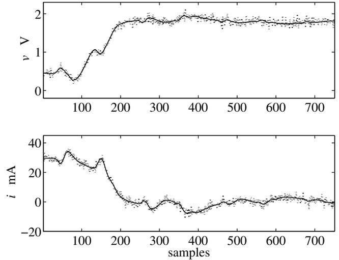
Fig. 8. Port voltage  $v(t)$  and current  $i(t)$  signals used for the estimation of submodel  $i_H$ , i.e., the solid thick signals in Fig. 5, with a superimposed gaussian white noise with standard deviation  $\sigma = 4\%$  of the voltage and current swing.
