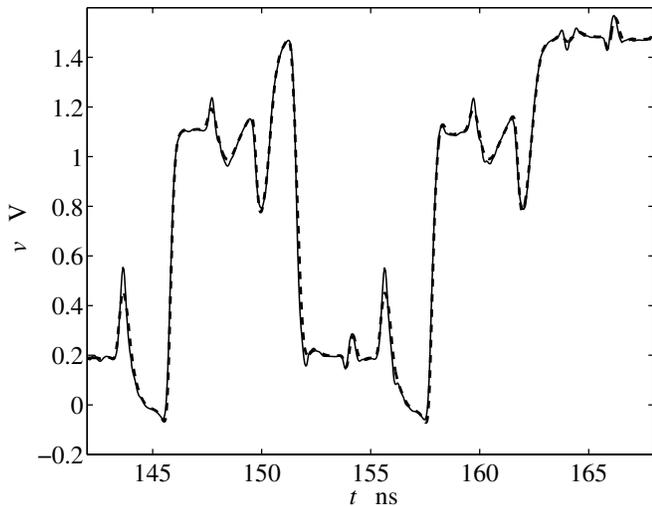
Fig. 7. Port voltage  $v(t)$  response computed for the example driver connected to an ideal transmission line load (characteristic impedance  $Z_0 = 50\Omega$ , time delay  $T_d = 1\text{ ns}$ ) loaded by the shunt connection of a  $100\Omega$  resistor and a  $5\text{ pF}$  capacitor.
