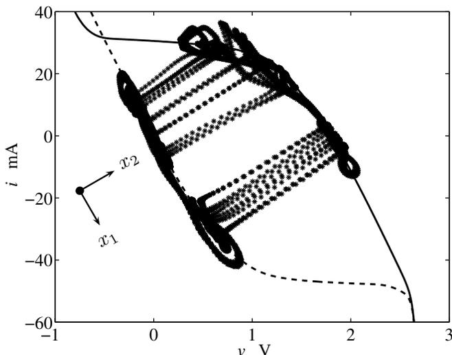
Fig. 4. Static characteristics of the example driver in fixed high state (solid thick line) and low state (dashed thick line) superimposed to the samples  $\{v(t), i(t)\}$  of the port transient response recorded while the driver is loaded by transmission-line load (star line).
