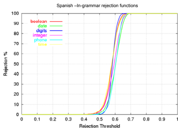
Figure 6: Rejection functions for the six built-in Spanish grammars using the normalized differential confidence.
