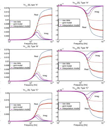
Fig. 3. Validation of the proposed interpolation scheme for two selected entries of the characteristic admittance  $\mathbf{Y}_c(s; \lambda)$ . In each panel, the upper and lower sets of curves correspond to grid points  $\lambda^{(k)}$  in the parameter space where raw data is available. Curves that are inbetween correspond to a validation point for the interpolated model.
