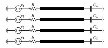
Fig. 5. Termination scheme for the generation of the eye diagram.
