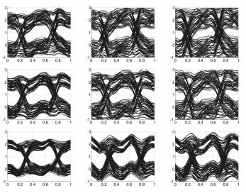
Fig. 7. Transmission eye sensitivity for the worst (synchronous clock) aggressors case, with single-ended signaling at 0.5 Gbps on a 30 cm interconnect. Rows from top to bottom correspond to d/w=2, 1.5, and 1 respectively. Columns from left to right correspond to w = 50, 100,  $150\mu$ m, respectively. Horizontal axis is normalized to twice the bit time. Vertical axis is voltage in Volts.
