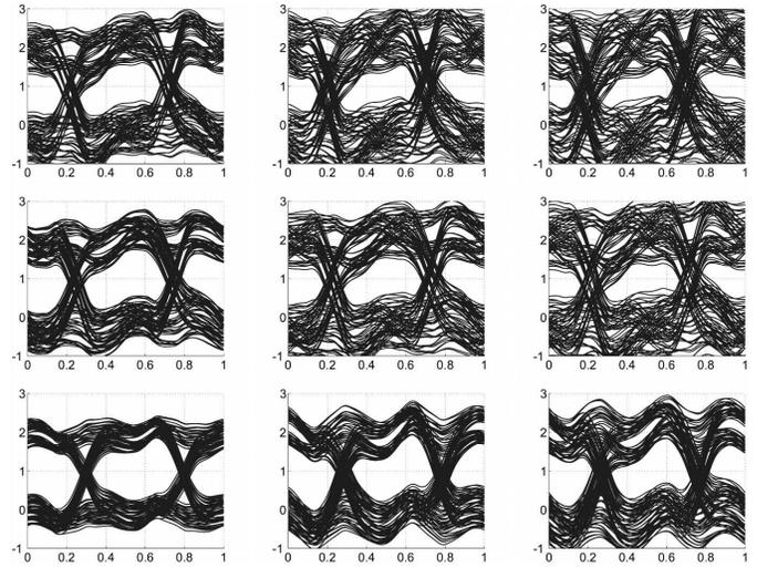
Fig. 7. Transmission eye sensitivity for the worst (synchronous clock) aggressors case, with single-ended signaling at 0.5 Gbps on a 30 cm interconnect. Rows from top to bottom correspond to  $d/w=2, 1.5,$  and  $1$  respectively. Columns from left to right correspond to  $w = 50, 100, 150\mu\text{m}$ , respectively. Horizontal axis is normalized to twice the bit time. Vertical axis is voltage in Volts.
