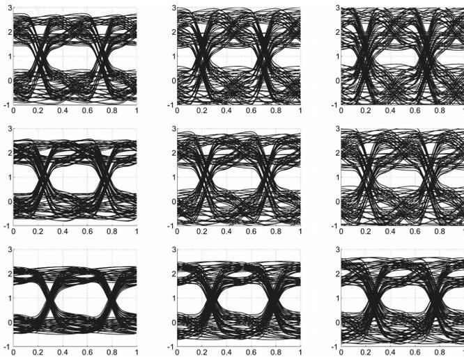
Fig. 6. Transmission eye sensitivity for the quiet aggressors case, with single-ended signaling at 0.5 Gbps on a 30 cm interconnect. Rows from top to bottom correspond to  $d/w=2, 1.5,$  and  $1$  respectively. Columns from left to right correspond to  $w = 50, 100, 150\mu\text{m}$ , respectively. Horizontal axis is normalized to twice the bit time. Vertical axis is voltage in Volts.
