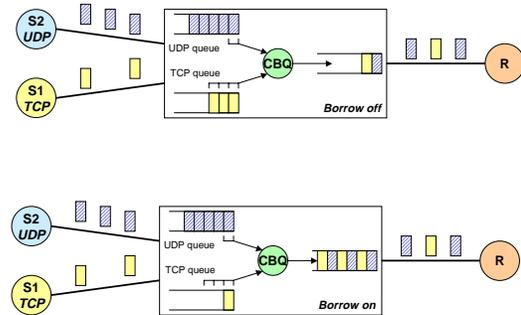
Figure 10: Different distribution of TCP packets when enabling borrow.
