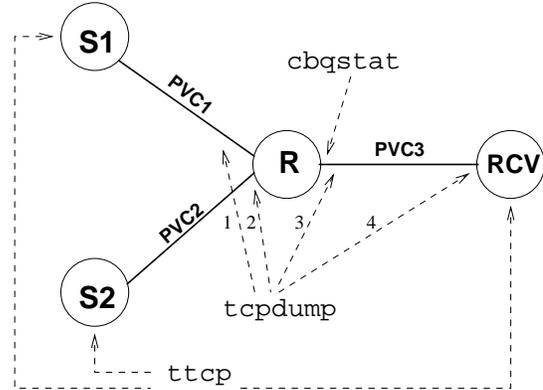
Figure 1: Network topology used in the experiments.
