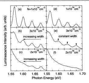
FIG. 3. Luminescence spectra calculated from the simulations (a)-(c) of the semiclassical Boltzmann equation and (d)-(f) of the semiconductor Bloch equations for various excitation densities N (same parameters as in the experiment).
