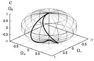
FIG. 2. (a) Simulated time evolution of the HQC gate 1 with  $\phi_1 = \pi/4$  and initial state  $|E^+\rangle$ . (b) Simulated time evolution of the HQC gate 2 with  $\phi_2 = \pi/2$  and initial state  $|E^+\rangle$ . (c) Simulated quantum evolution of gate 2 in the control parameter manifold  $(\Omega^-, \Omega^+, \Omega^0)$ . In these simulated experiments we have chosen  $\Omega^{-1} = 50$  fs and  $T_{ad} = 7.5$  ps (see text).
