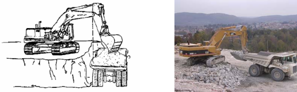
Figure 5. Example of optimal placement of the shovel and truck.
