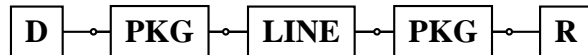
Figure 1: Main parts of a generic board-level interconnected system. D : drivers; PKG : packages; LINE : interconnect; R receivers.
