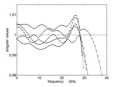
Figure 4: Singular values of the scattering matrix of the model of Fig. 3 vs. frequency.
