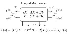
Figure 1: State-space based macromodeling. Arrays Y and U collect input and output wave variables at all ports.
