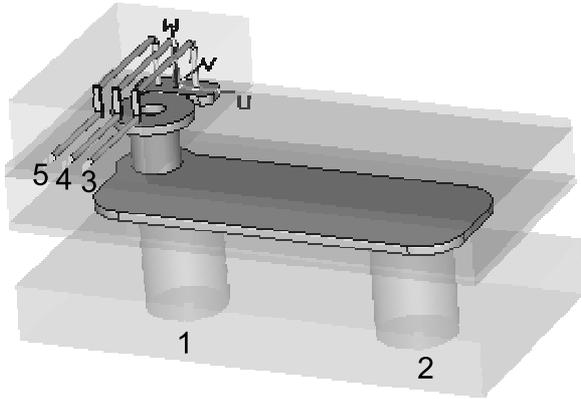
Figure 2: Five-port element used to test pole estimation via 4SID for real modeling problems. The hot terminals of the ports are indicated by the numeric labels.
