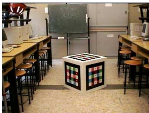
Figure 68: reference points on a calibration object, and their position on the image plane
