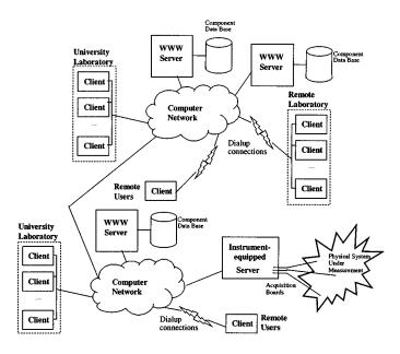
Fig. 1. Distributed system architecture.
