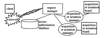
Fig. 4. Software architecture of the instrument-equipped server.
