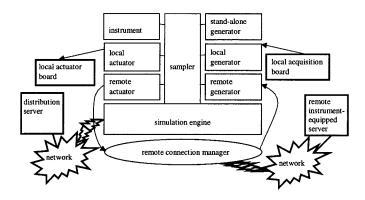
Fig. 2. Client software architecture.
