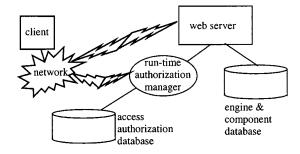
Fig. 3. Software architecture of the distribution server.
