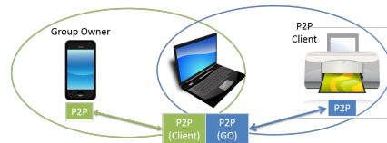
Fig. 2. Communication between two Wi-Fi Direct groups.
