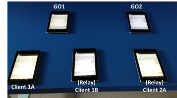
Fig. 4: The placement of the five tablets, forming two Wi-Fi Direct groups: 3 devices in the left group and 2 devices in the right group.
