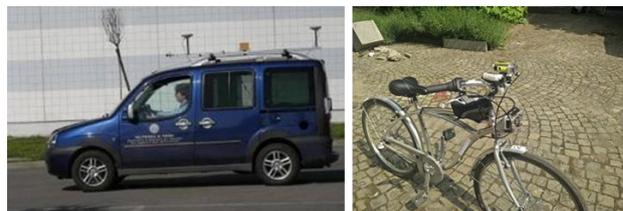
Figure 2. Mobile Mapping System on car and bicycle
