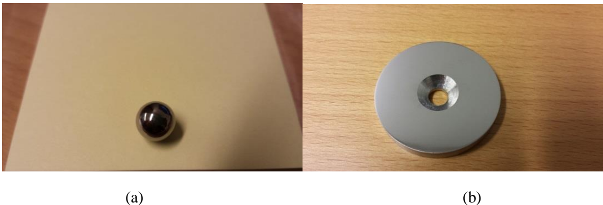
Figura 3.311 - Sfera in WC-Co (a) e disco in Ti-6Al-4V (b)
