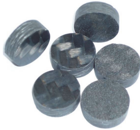
Figure 1. Specimens for the creep compression tests.
