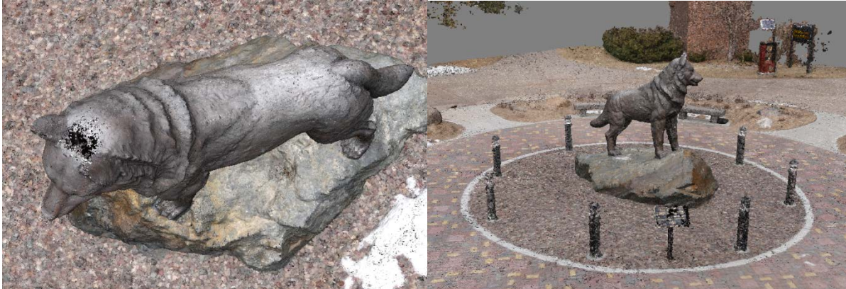
Figure 10. Dense cloud images. Left is result of needing more images. Right is whole scene.
