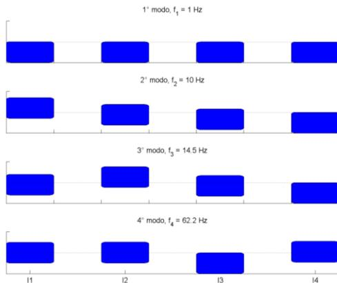
Fig. 4 – Natural frequencies and mode shapes computed from the simulation model.
