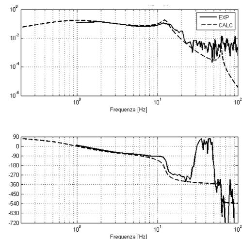
Fig. 10 - FRF  $\dot{\theta}_{M1}/T_{M2}$ : modulus (top) and phase [°] (bottom).
