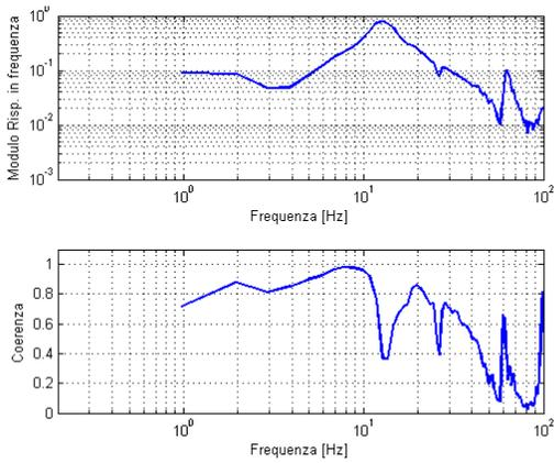
Fig. 6 – FRF  $\dot{\theta}_{M2}/T_{M2}$ : modulus (top) and coherence function (bottom).
