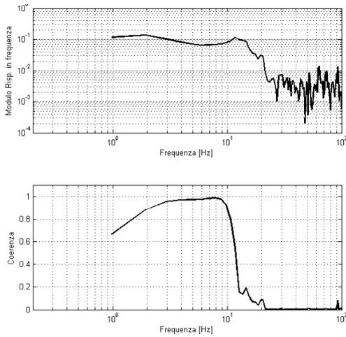
Fig. 7 - FRF  $\dot{\theta}_{M1}/T_{M2}$ : modulus (top) and coherence function (bottom).
