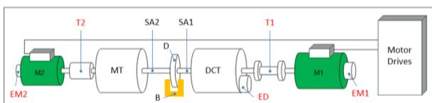
Fig. 2 – Transmission test bench layout. M1, M2: electric motors; EM1, EM2, ED: speed sensors (encoders); T1, T2: torque sensors; B: disk (D) brake; SA1, SA2: half shafts.
