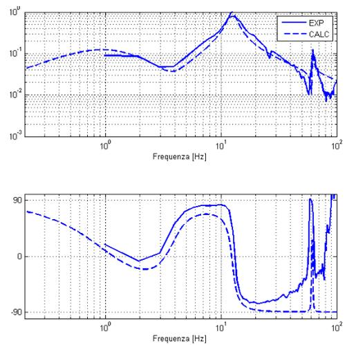
Fig. 9 – FRF of  $\dot{\theta}_{M2}/T_{M2}$  : modulus (top), phase [°] (bottom)
