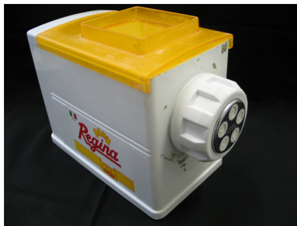
Figure 1. The extruder used for manufacturing bucatini and maccheroni .
