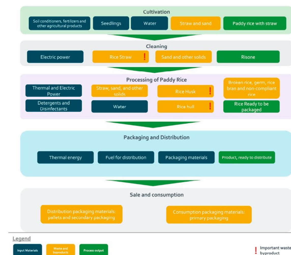
Figure 8. Flow diagram of the main supply chain steps with the main inputs (in blue), waste and by-products (in yellow), and products (in green), as reported both in the focus group sessions, as well as the project report for the Rice supply chain [53].
