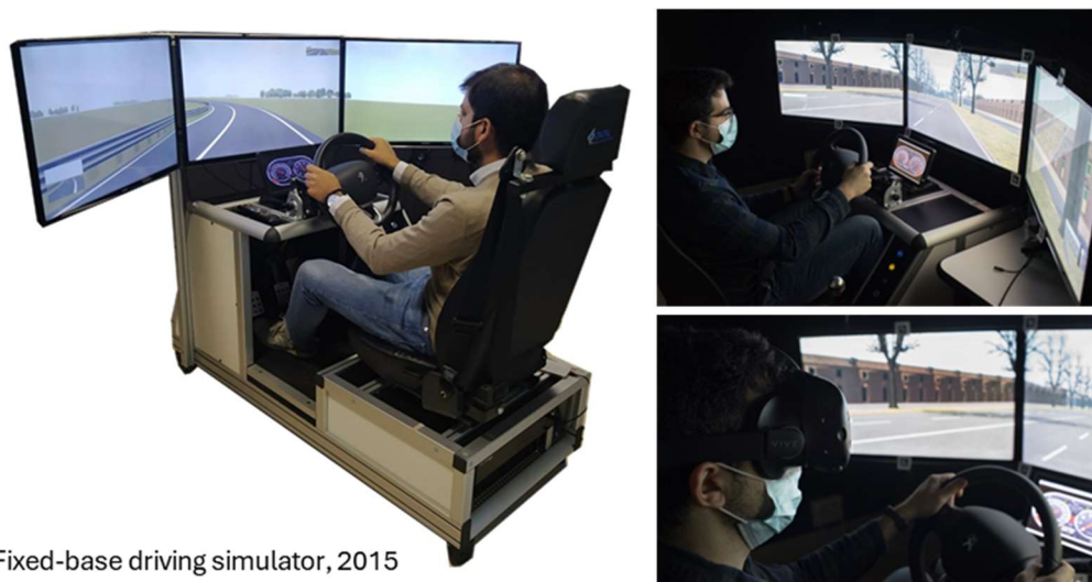
Figure 11: The fixed-base driving simulator (acquired in 2015) at the RSDS Lab is equipped with a visual system that operates using either a three-screen setup or a virtual reality (VR) headset. For the experiments described in this thesis, the three-screen vision system was used.
