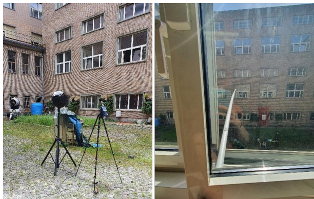
Figure 3. Picture of the source and receivers in the courtyard (right) and façade receivers positions (left)
