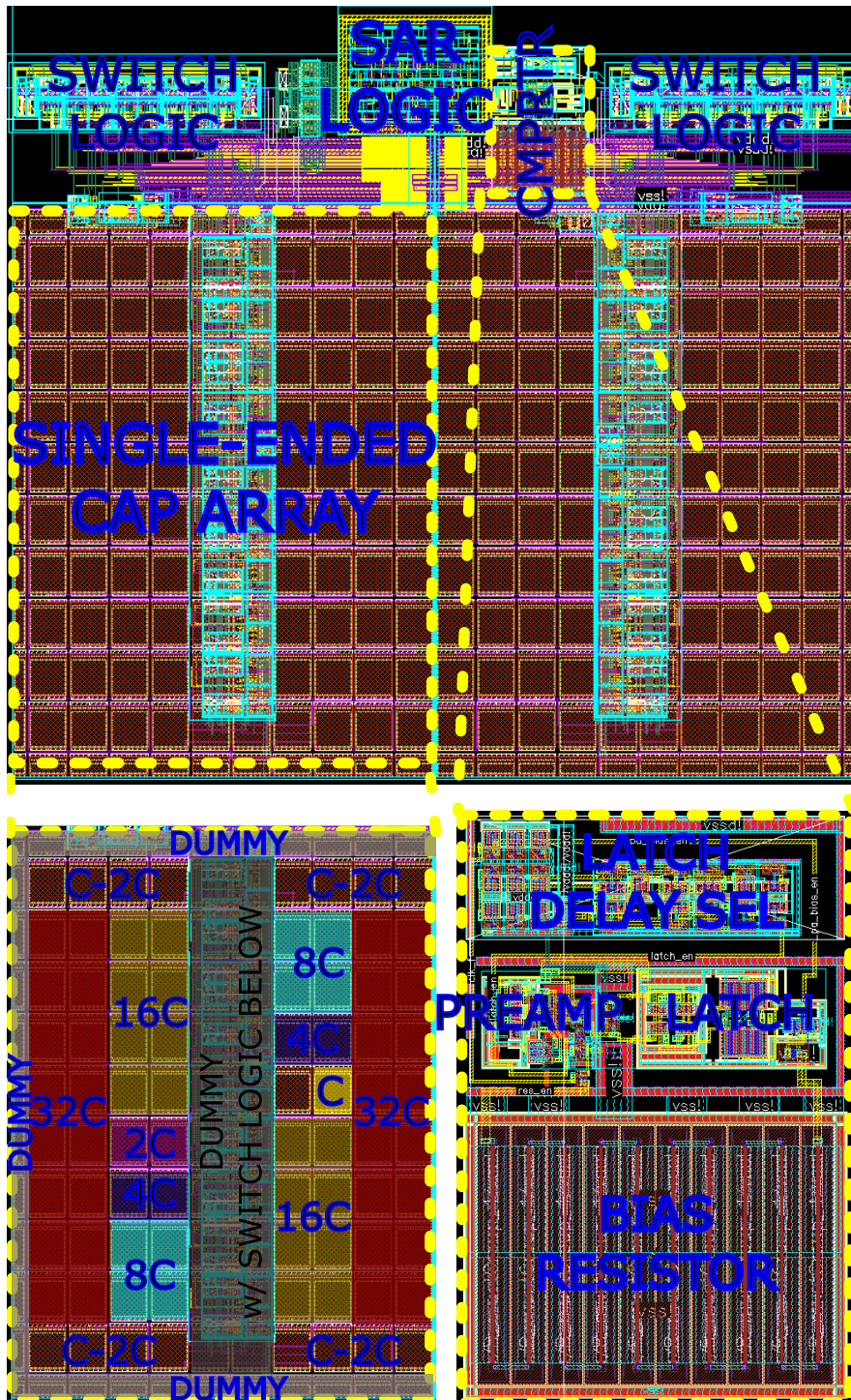
Fig. 3.21 (a) Layout of a single differential CS encoder. (b) Common centroid layout of the capacitor array, with dummy elements on the outer boundary and dummy elements in the middle to allow a closer placement of the driving switches to the capacitive elements. (c) Layout of the dynamic comparator.
