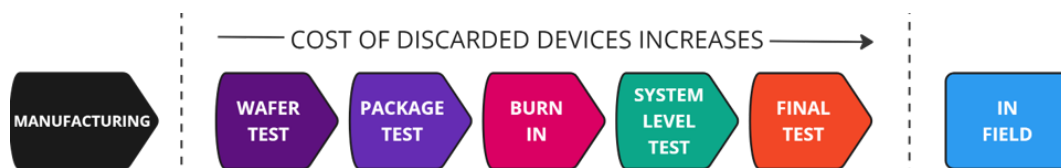
Fig. 2.1 Manufacturing testing flow for safety critical sectors. As it can be noted catching malfunctions at the early stages of manufacturing reduces costs, as next stages won't be applied to discarded dies.
